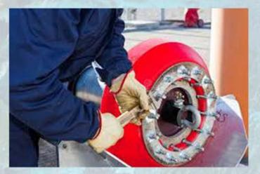
Smart pigging provides a number of advantages over traditional forms of pipeline inspection. It allows pipelines to be cleaned and inspected without having to stop the flow of product. It also allows the a pipeline to be completely inspected without having to send inspectors down its entire length. Finally, it provides cleaning and inspection services at the same time, saving companies both time and money.
